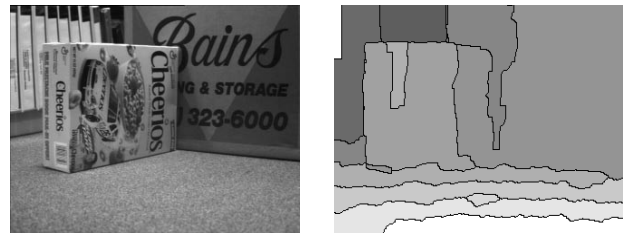
Figure 1: LEFT: An image from a stereo pair. RIGHT: The disparity map, with region boundaries overlaid, computed by the algorithm of [6], which searches over quantized disparities. The scene geometry is poorly captured by this output.
