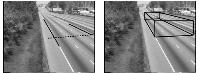
Fig. 3. Camera calibration. (Left) User draws three lines—(solid) two along the edges of the road and (dashed) one perpendicular to the direction of travel. The lines can be of arbitrary length. (Right) Three-dimensional detection zone is automatically computed.
