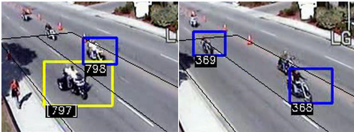
17 18 FIGURE 10 Examples of miscounted motorcycles for site 2
