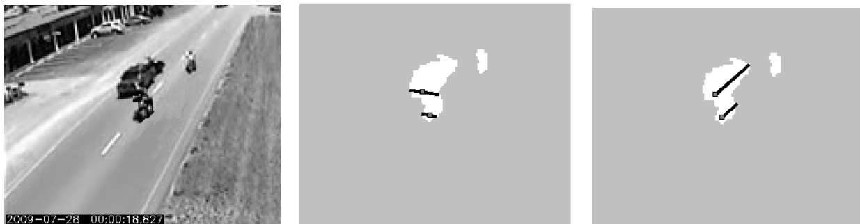
FIGURE 3 Measuring the width (middle) and length (right) of tracked vehicles (left)
