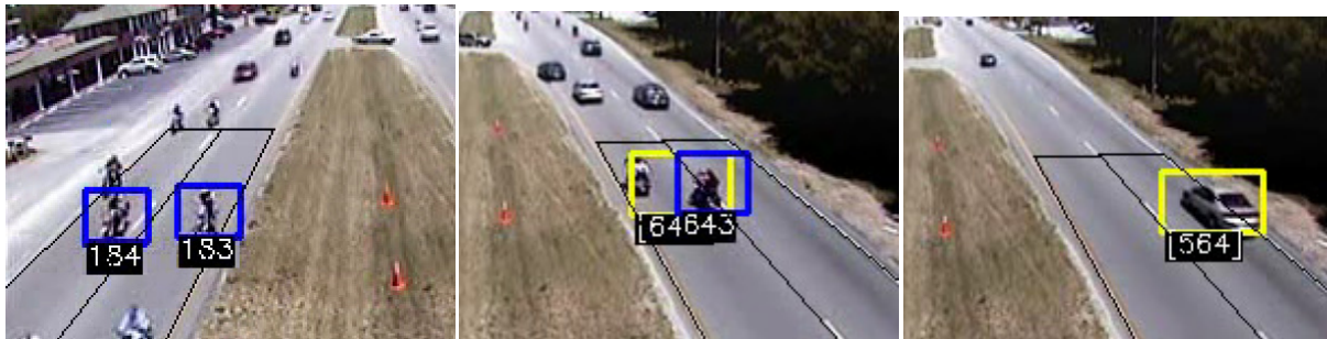
FIGURE 8 Examples of miscounted or incorrectly classified vehicles
