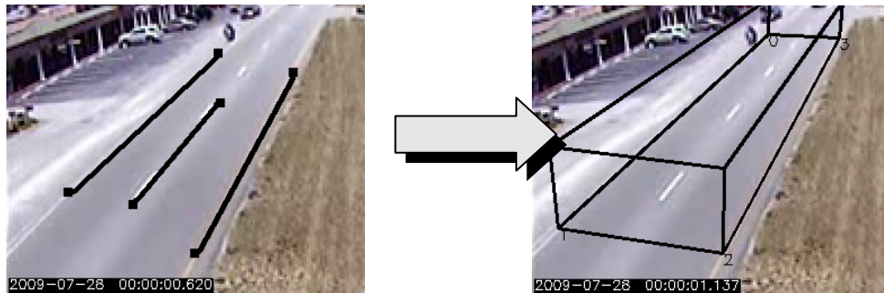
FIGURE 2 “Six-click” calibration procedure using lane lines
