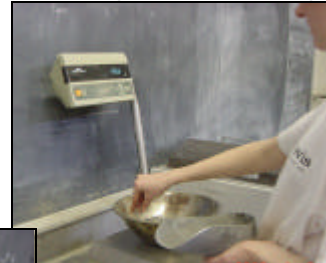
Then it is measured into the bowls by weight to be later combined with modified rubber binder.
