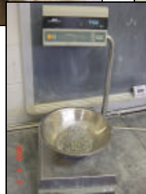
Then it is measured into the bowls by weight to be later combined with modified rubber binder.
