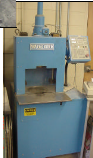
Once the ingredients are mixed at the proper temperature and cured in the oven, the sample is compacted using the gyratory compactor.
