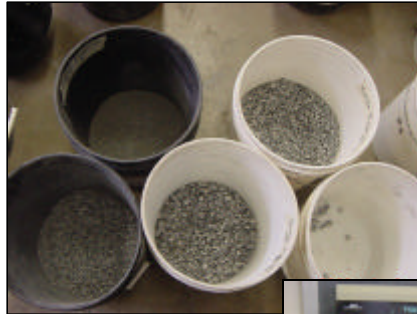
Aggregate is sieved to separate into various sizes.
