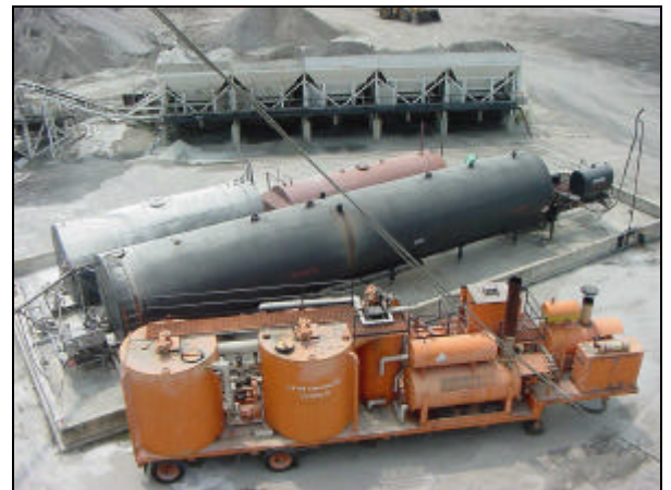
Figure 1: Portable blending equipment such as the piece in the foreground was used for two of the projects.
