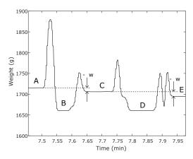
Fig. 3: Scale data generated while a sandwich is picked up and returned to the scale twice. The weight of food consumed can be found based on the change in weight values identified in the figure.
