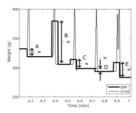
Fig. 2: The effect of down-sampling at .33 Hz to measure bite weights.
