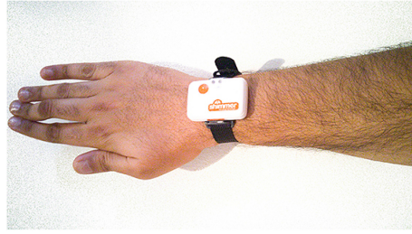
Fig. 5. The Shimmer3 sensor mounted on the wrist. This sensor was used for data collection in the pedometer [16] and free-living eating activity datasets (this work). The custom IMU sensor in the cafeteria dataset [25] is mounted in the same manner.
