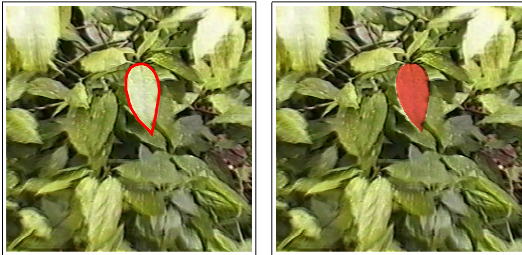
Figure 1.14: Automated video editing. Tracking the outline of a foreground object allows it to be separated automatically from the background, and manipulated as desired, a special effect which can otherwise only be achieved by “blue-screening” from specially prepared footage.
