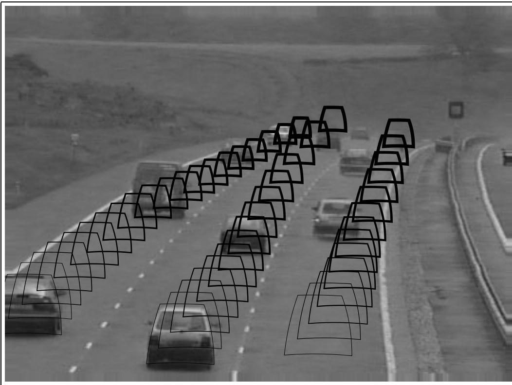
Figure 9.13: Dynamical model for traffic. Three simulated trajectories for an ARP set up to represent the traffic pattern, each initialised with a velocity in shape-space corresponding to translation along the road, coupled with shrinkage consistent with perspective scaling. Translational parameters are \beta = f = 0 (constant-velocity) with \gamma_0 = 35 \text{ pixel}\cdot\text{s}^{-3/2} , allowing the paths to veer over longer times. Affine deformations are critically damped ( f = 0 ) with a long time-constant ( 1/\beta = 10 \text{ s} ), and largely deterministic ( \bar{\rho} = 2 \text{ pixels} ), allowing the outline to shrink steadily. Contours are plotted here at intervals of 200 ms.
