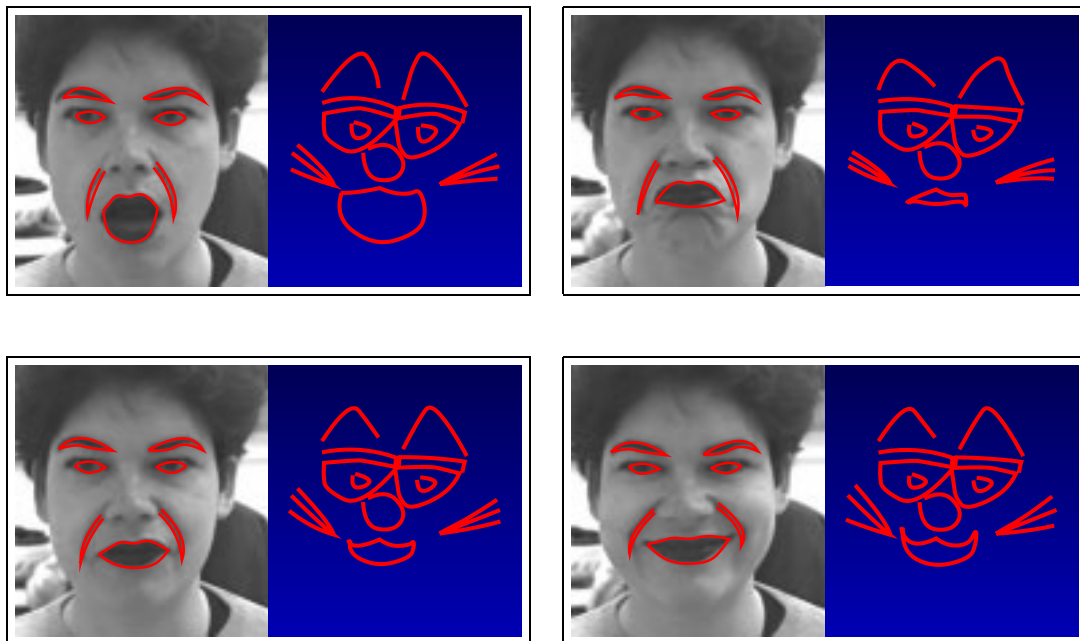
Figure 1.2: Actor-animated cat. Tracked facial motions drive input channels to a cartoon cat, programmed with some exaggeration of expression. (Figure courtesy of Benedicte Bascle, Ben North and Julian Morris.)
