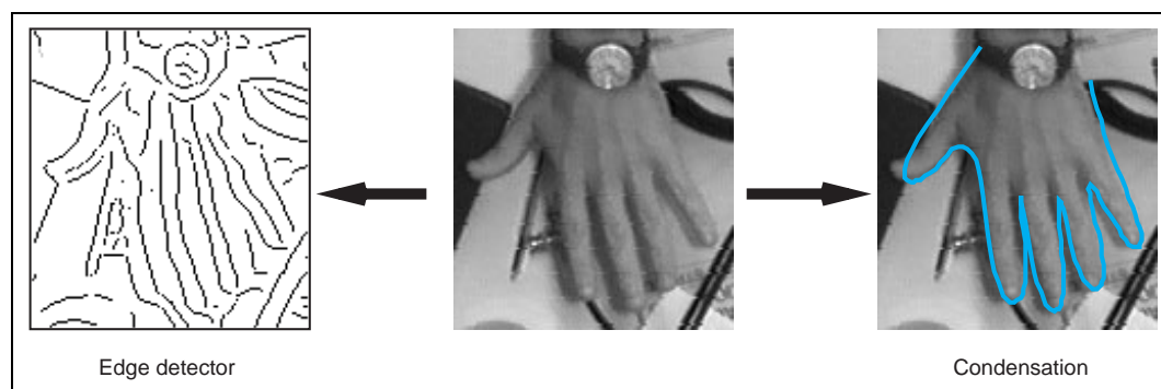
Figure 12.15: Severe clutter. Detail of one field from the test sequence shows the high level of potential ambiguity. Output from a directional Gaussian edge detector shows that there are many clutter edges present as potential distractors.
