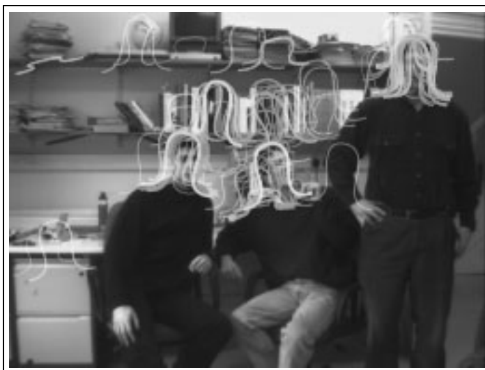
Figure 12.4: Sample-set representation of posterior shape distribution for a curve with parameters \mathbf{X} , modelling a head outline. Each sample \mathbf{s}^{(n)} is shown as a curve (of varying position and shape) with a thickness and intensity proportional to the weight \pi^{(n)} . The prior is uniform over translation, and a constrained Gaussian in the remainder of its affine shape-space. (Figure taken from (MacCormick and Blake, 1998).)
