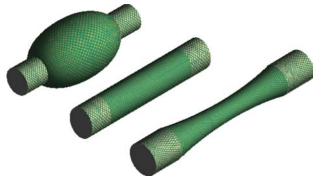
Figure 9. Pneumatic air muscle actuators with a mesh angle of less than 54^{\circ}44' contract on pressurisation (left), with a mesh angle of 54^{\circ}44' neither extend nor contract (middle), and of greater than 54^{\circ}44' extend on pressurisation (right).
