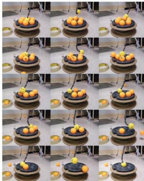
Figure 13. Removal of balls from a tray. Time (approximately 1 minute) evolves from the top to the bottom row, left to right in each row. The experiment demonstrates the ability of a discrete control strategy, exploiting impact dynamics in selectively manipulating objects in complex environmental fields.
