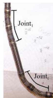
Figure 2. Tendril continuum manipulator prototype. The diameter of the backbone is 0.4 inch. The joints labelled (neither is fully flexed in image) have a length of 3.25 inches. The overall length of the tendril used in experiments is 18 inches.
