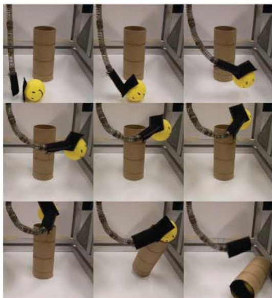
Figure 10. Acquiring a payload and manipulating it into a hole. The diameters of the (ping pong) ball and the (toilet roll core) tube are approximately 1 inch. Time (approximately 10 seconds) evolves from the top to the bottom row, left to right in each row. The experiment demonstrates the ability of the robot to carry and manipulate small objects if equipped with a small magnet or gripper at the tip.
