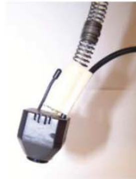
Figure 8. Tendril tip with an externally powered camera.
