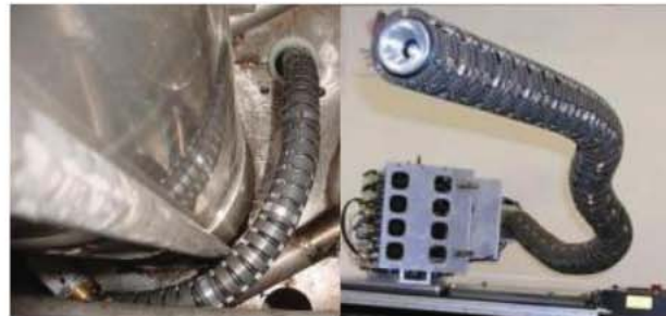
Figure 17. Commercially manufactured snake-arm robots from OC Robotics. Adapted from [6]. Applications include repair in nuclear reactors (left image) and inside airplanes.
