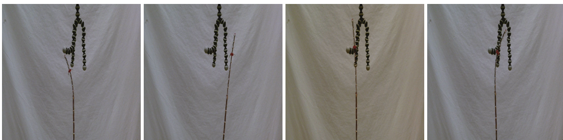
Figure 7. Circumnutation with tendril robot ending in achieving environmental attachment.
