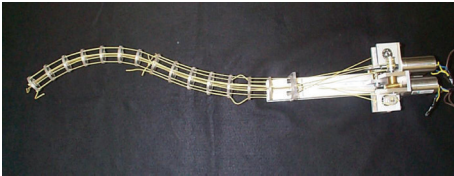
FIGURE 4: Tendon-based continuum robot with incompressible flexible rod core.
