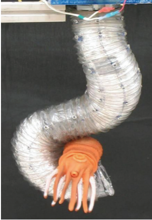
FIGURE 3: Air-Octor Continuum robot. This two-section, six-degree-of-freedom robot bends a pneumatically inflated core tube using six tendons.
