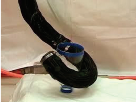
FIGURE 1: A continuum robot grasping and manipulating a fragile (glass) object, using its compliant backbone to adapt to the object's shape.
