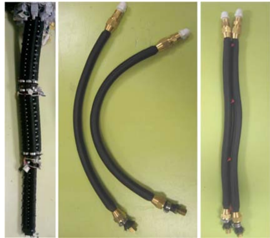
Fig. 2. Octarm VI, individual actuators and planar equivalent prototype
