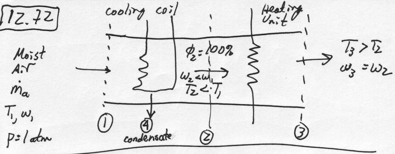
$$T_1 = 26^\circ\text{C} \quad \phi_1 = 0.80 \quad \dot{V} = 0.47 \text{ m}^3/\text{s}$$
