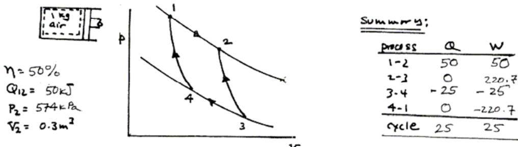
ENGR. MODEL: 1. The system shown in the schematic consists of air modeled as an ideal gas. 2. Volume change is the only work mode.
