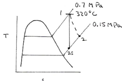
ENGR. MODEL: (1) The control volume shown in the figure is at steady state. (2) For the control volume,  $Q_{cv} = 0$ , and potential energy effects are negligible.
