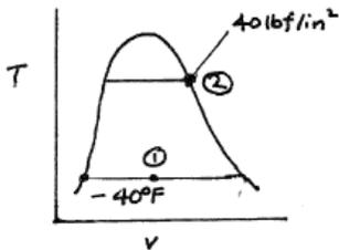
Table A-10E at  $-40^\circ\text{F}$ :  $h_f = 0$ ,  $h_{fg} = 95.82 \text{ Btu/lb}$
