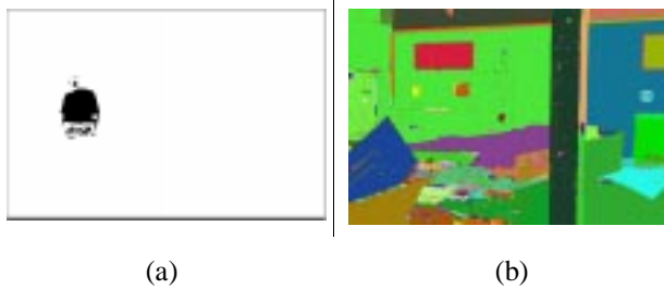
Figure 4. (a) Active blob in newlab2 sequence which represents a partially occluded moving person. (b) Flood-filled static blobs from same sequence are monitored for consistency.
