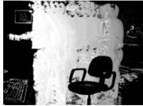
Figure 3. This shows a motion history image (MHI) of a moving person in a scene. Note how occlusion information allows us to identify the chair and its location in front of the person. For more information on motion history images see [3].
