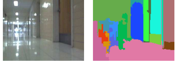
Fig. 3. LEFT: A door with a kick plate. RIGHT: The segmentation of the image using the efficient minimum-spanning-tree algorithm [6], in which the kick plate is identifiable as the olive green region at the bottom of the door.
