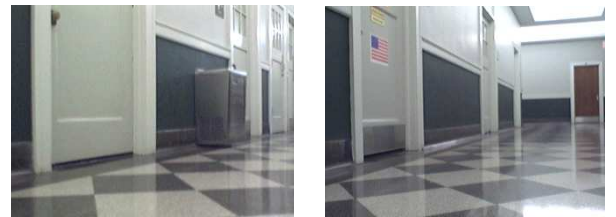
Fig. 15. Doors successfully detected by our algorithm. Note the variety of door widths, door and wall colors, relative pose of the door with respect to the robot, floor texture, and lighting conditions. Distant doors are not considered by the algorithm.
