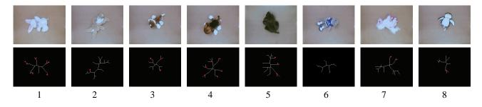
Fig. 10. TOP: Images of the individual objects used for creating a database of previously encountered items. BOTTOM: The final skeletons of the objects with revolute joints automatically labeled (red dots).
