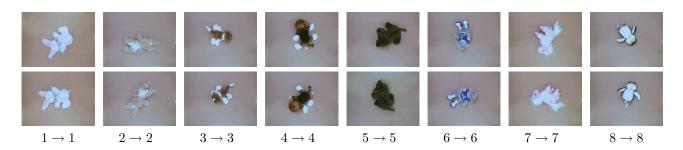
Fig. 11. Results from matching query images obtained during a second run of the system (top) with database images gathered during the first run (bottom). The numbers indicate the ground truth identity of the object and the matched identity. All of the matches are correct.
