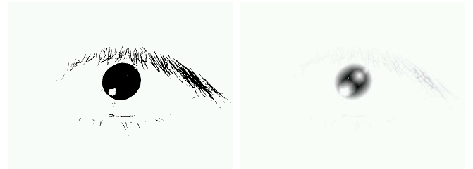
Fig. 3. Eye image after thresholding (left) and chamfer operations (right).
