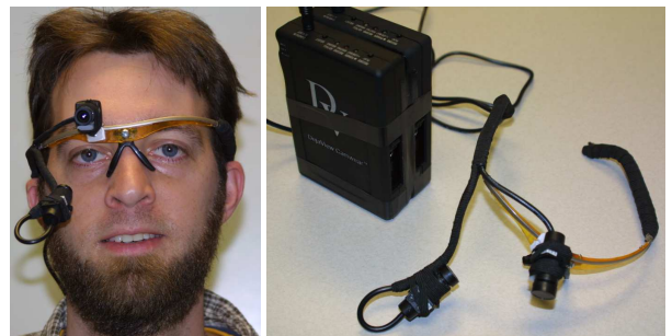
Figure 2: Our do-it-yourself wearable eye tracker from relatively inexpensive ( \sim \$700) off-the-shelf components.
