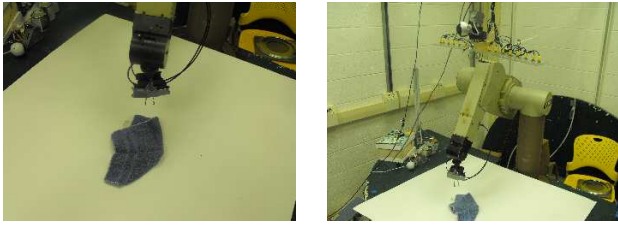
Fig. 2. The robot system used for flattening a piece of clothing, in this case a washcloth: One PUMA manipulator and one Logitech Quickcam 4000.
