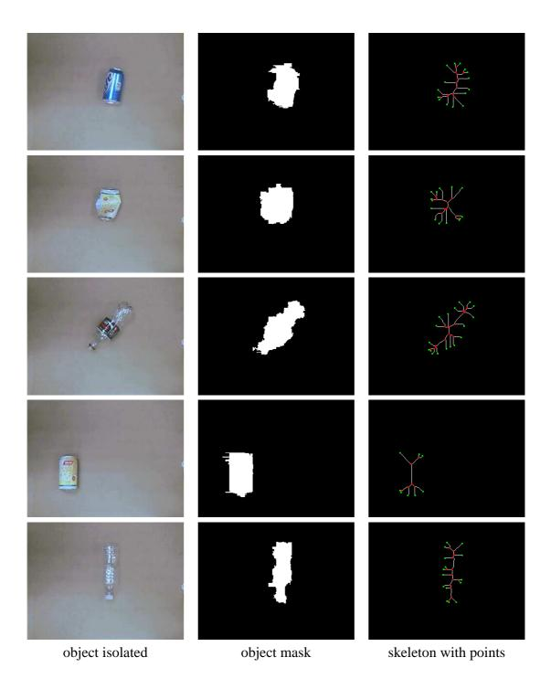
Figure 4.13: Example of a recycling experiment containing a pile of five plastic and metal objects that were individually separated and examined. From left to right: The image taken after the object has been picked up and separated, the binary mask of the isolated object, and the skeleton with the intersection points and end points labeled. Time flows from top to bottom, showing the progress as each individual object is examined.
