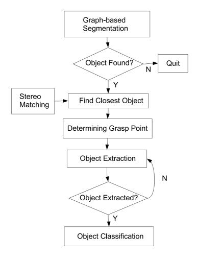
Figure 2.1: Overview of our system for vision-guided extraction of a pile of unknown objects.
