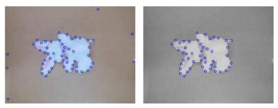
Figure 3.4: LEFT: KLT features selected in the whole image. RIGHT: Features that are located within the region selected by graph-based segmentation.
