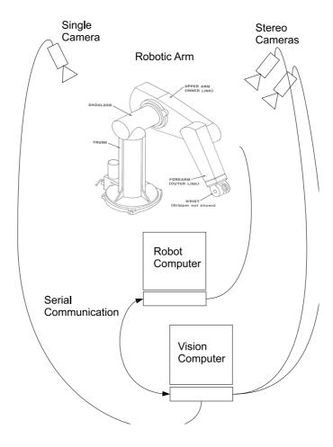
Figure 4.1: The setup and connection of the robot computer, main computer, and three webcams.
