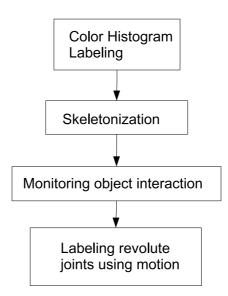
Figure 3.1: Overview of our system for manipulation-guided classification of a pile of unknown objects.
