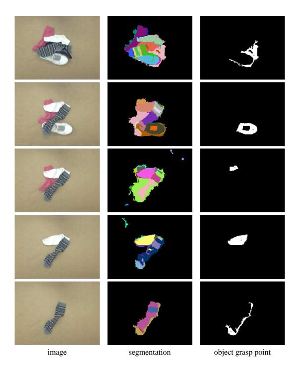
Figure 4.16: Example of a service robot experiment containing a pile of socks and shoes that were individually separated and examined.
