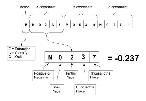
Figure 4.4: The serial communication format.
