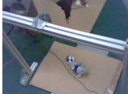
Figure 1.1: The proposed setting for manipulation-guided sensing. Left: A robotic arm interacts with a pile of unknown objects (stuffed animals) to segment the individual items one at a time. An overhead stereo pair of cameras (Logitech QuickCam Pro webcams) is not shown. Right: The system then learns about each object's characteristics by automatically isolating it from the pile and interacting with it. A third overhead camera is used for sensing the isolated object.
