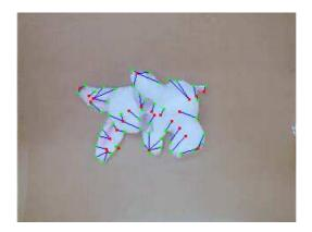
Figure 3.7: Example of mapping feature points to the nearest intersection point. The red dots represent the intersection points (possible revolute joints) of the skeleton. The green dots represent the feature points gathered by KLT. The blue lines connecting various points together represents the mapping of the feature point to the closest intersection point of that feature.
