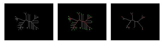
Figure 3.8: LEFT: The original skeleton. MIDDLE: Skeleton with intersection points and end points labeled. RIGHT: Revised skeleton after multiple interactions. The red dots represent the intersection points (possible revolute joints) of the skeleton. The green dots represent the end points (interaction points) of the skeleton.
