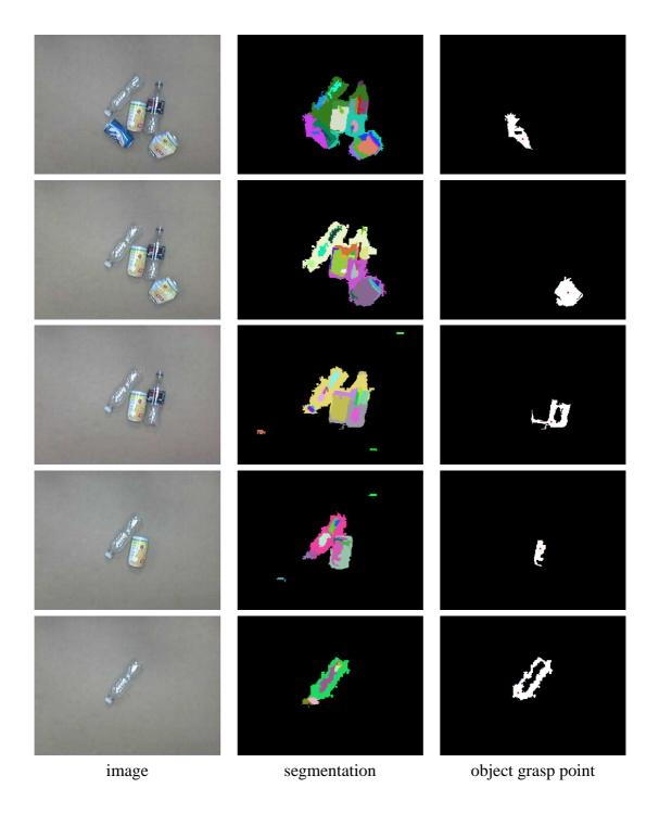
Figure 4.12: Example of a recycling experiment containing a pile of five plastic and metal objects that were individually separated and examined.
