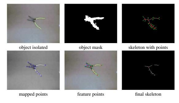
Figure 4.20: Example of comparing our approach to that of related work in [12]. From top left to bottom right: The image taken after the object has been picked up and separated, the binary mask of the isolated object, the skeleton with the intersection points and end points labeled, the feature points gathered from the isolated object, the image after mapping the feature points to the intersections points, and the final skeleton with revolute joints labeled.
