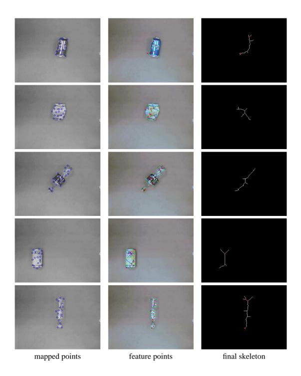
Figure 4.14: Continuing the same experiment from Figure 4.13. From left to right: The feature points gathered from the isolated object, the image after mapping the feature points to the intersections points, and the final skeleton with revolute joints labeled. Time flows from top to bottom, showing the progress as each individual object is examined.
