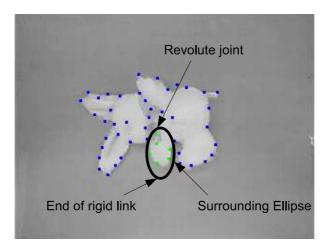
Figure 3.6: Example of grouping feature points to locate revolute points near the endpoints of the major axis.
