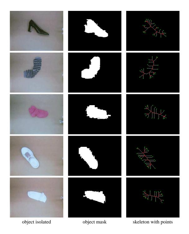
Figure 4.17: Example of a service robot experiment containing a pile of socks and shoes that were individually separated and examined. From left to right: The image taken after the object has been picked up and separated, the binary mask of the isolated object, and the skeleton with the intersection points and end points labeled. Time flows from top to bottom, showing the progress as each individual object is examined.
