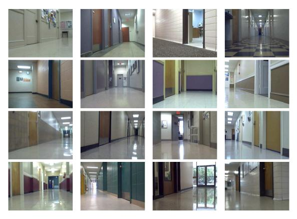
Figure 1.1: Typical corridor images are shown. Strong reflections, shadows, dark areas, and low-contrast in color are commonly seen, which bring difficulties to vision-based mobile robot navigation.
