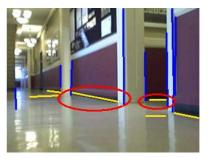
Figure 2.7: Horizontal and vertical line segments detected in two images. The red ellipses highlight the horizontal segments with the highest bottom score, due to their proximity to the bottom endpoints of nearby vertical line segments (Best viewed in color).
